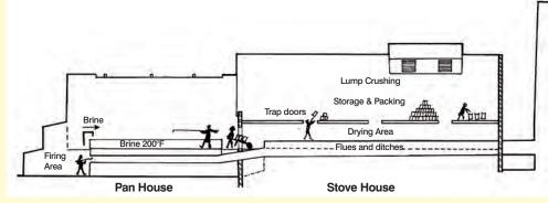
Open pan salt works made fine salt and block salt in a Pan House with an attached Stove House. Coal was burnt under the iron pan. Salt was skimmed into boxes and barrowed into the Stove House. Flues carried heat and fumes from the furnace underneath the Stove House to a chimney. Rising heat dried the salt when it was 'lofted' to the warehouse floor above.
