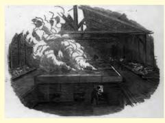
A fine pan described in the Illustrated London News 1850. Fishery pans could be much larger and made coarser crystals in pans set up outdoors to replicate 'Bay Salt'.
